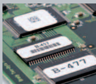
Circuit Board Labeling
